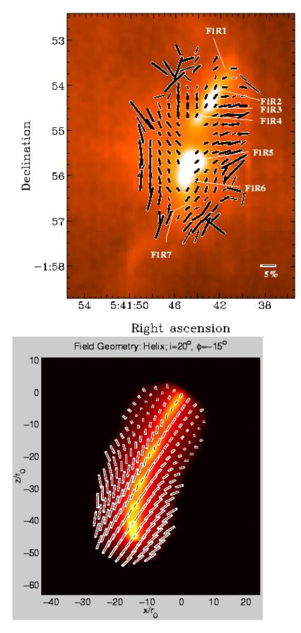
(Figure 1 left) Using the imaging polarimeter for the Submillimeter Common User Bolometric Array at the James Clerk Maxwell Telescope, we have detected polarized thermal emission at 850 um from dust toward the NGC 2024 star-forming core system. Here we show the 850 um dust emission as a ``grey"-scale, on which are plotted the 12"-binned polarization vectors. Vectors are plotted where I>0.001 V, p>1%, dp<1.5% and p/dp>4. Bold vectors
