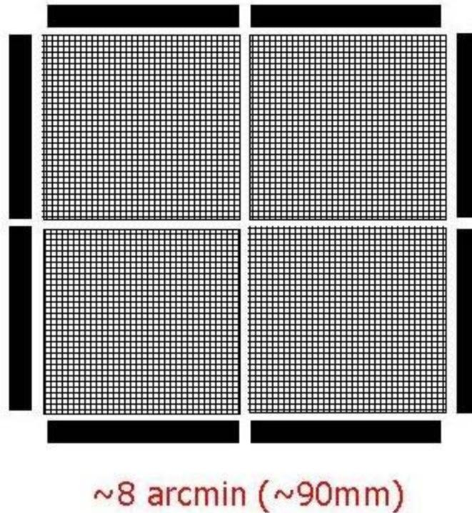
*FIGURE 2: Array focal plane layout showing the 4 sub-arrays butted together.*
