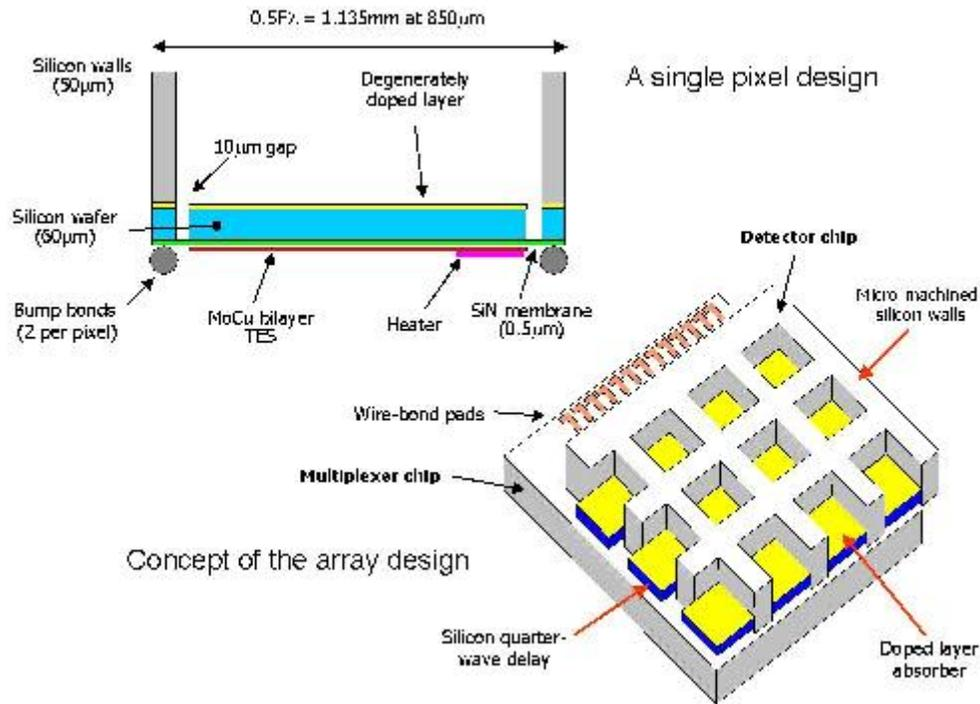
FIGURE 1: (a) Single pixel schematic diagram (b) Concept of the array architecture design
