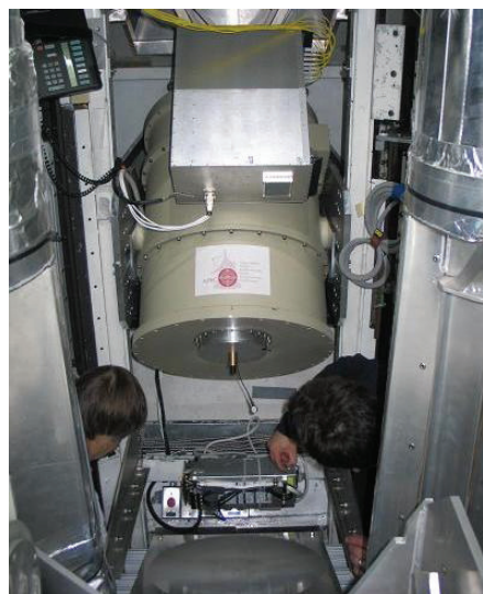
Figure 1. — Installation and optical alignment of AzTEC in the JCMT receiver cabin.
