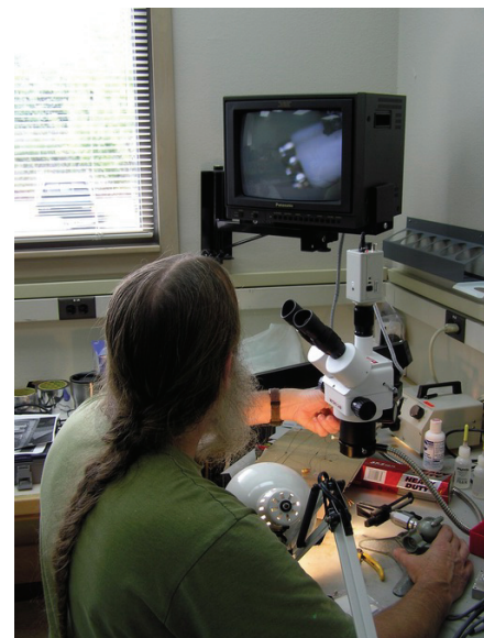
Figure 5. — Ken Brown 'enjoying' several weeks of use of a stereo microscope to solder wires and connectors for installation inside the cryostat.
