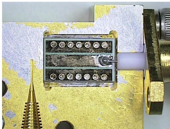
The IF Transmission Line to SMA Connector
