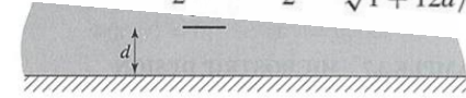
FIGURE 3.26 Equivalent geometry of quasi-TEM microstrip line, where the dielectric slab of thickness d and relative permittivity \epsilon_r has been replaced with a homogeneous medium of effective relative permittivity, \epsilon_e .
