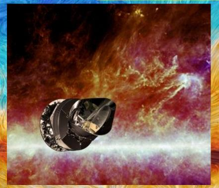
Planck is a third generation space based cosmic microwave background experiment, operating at nine frequencies between 30 and 857 GHz
