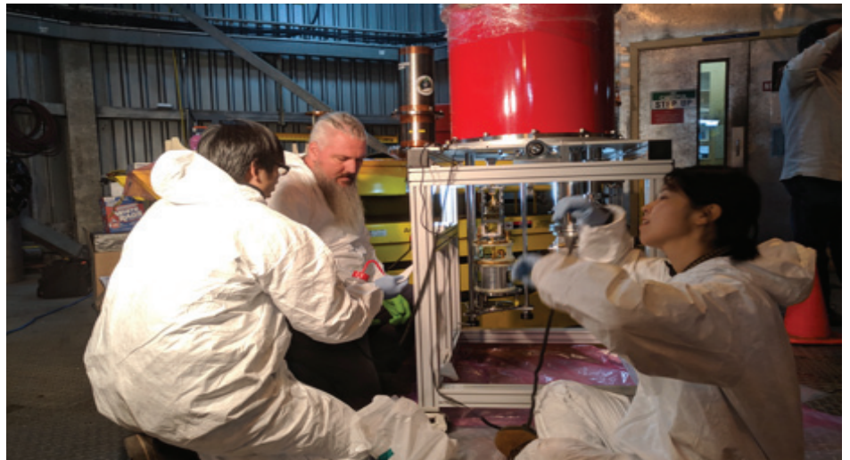
Figure 22: Kuan-Yu Liu, Jason Fleck, and Izumi Mizuno insert the cold cartridge little by little into the dewar by carefully checking insert angle.
