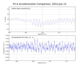
Amplitude correlates with GNIRS coldhead stroke parallel to X axis. 12 Hz amplitude absent parallel to Y.
