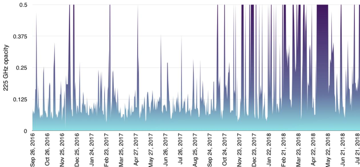
Figure 3. Measured opacity (225 GHz) via the WVM since September 2016.
