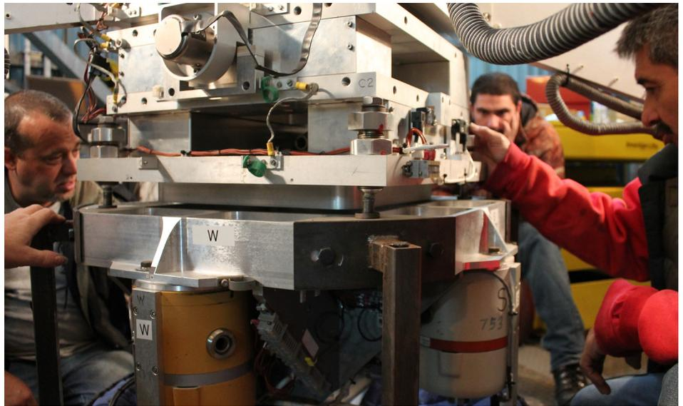
Figure 19. Neal Oliveira, Simeon Johnson, and Vernon DeMattos reattaching the chopper unit to the tables of the SMU. Photo by Kevin Silva
