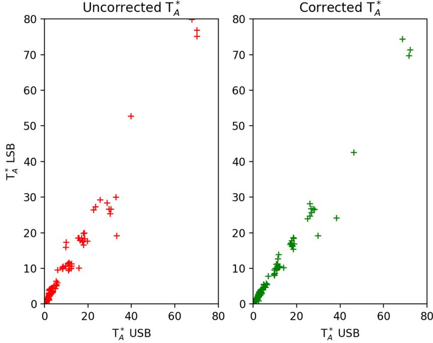
Figure 4:  $T_A^*$  in the LSB as function of  $T_A^*$  in the USB. The plot to the left shows the correlation before applying the correction and the right plot the correlation after applying the correction for the sideband gain. There is a clear improvement but as can be seen some discrepancies remains.
