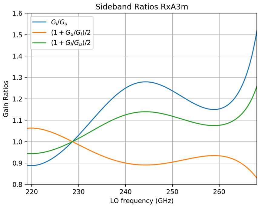
Figure 5:  $G_l/G_u$ ,  $(1 + G_l/G_u)/2$ ,  $(1 + G_u/G_l)/2$ . The raw4 fit from 1 has been used in this plot.
